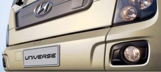
Protrusion typed front bumper and fog lamp
