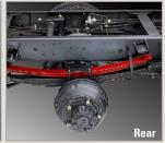
□ High capacity axle and leaf suspension Generous 320 mm x 75mm brake linings (with The higher capacity axle and leaf suspension of HD45 exhibits outstanding durability and rigidity and maximize load carrying performance.
